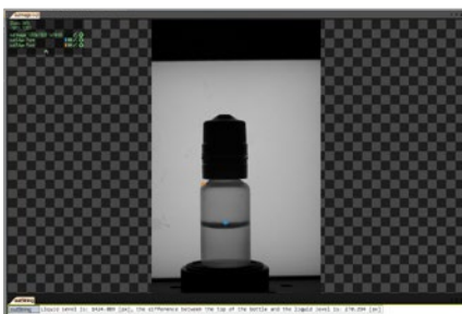
FabImage Studio can be used to create a software indicating the liquid level in just a few steps.
