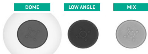
Various illumination geometries provide different kind of information on the object. Here, a mixed illumination is the best choice.
